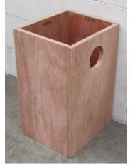
2. Align the bottom of one side with the base and attach the screws.
