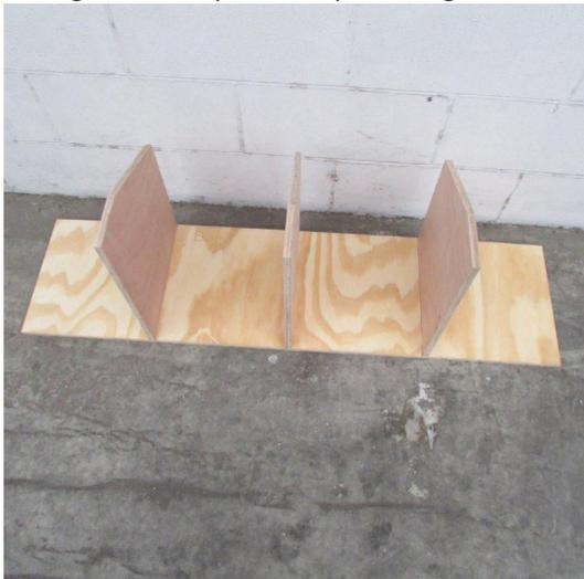
Attach the back to the base and the short end of the dividers.
